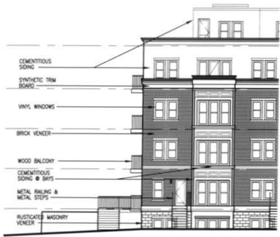
BUILDING CORNER ELEVATION 0 5 10 20'
